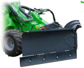
The Avant snow plow is a versatile attachment for snow removal. It consists of two independently hydraulically adjustable blades. Angle of the blades can be adjusted with a switch from the driver's seat. Both blades have a
