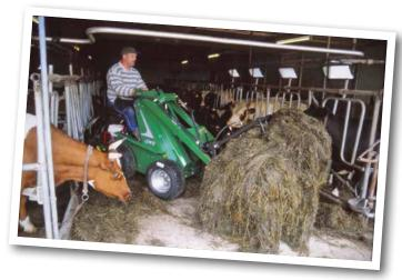
In its early days Avant was advertised solely as a machine for feeding livestock. The machine was strong and agile, could move in confined spaces and most importantly, made the heavy work much easier.
