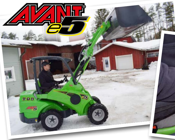
The 60 cm telescopic boom brings more reach and lifting height.
