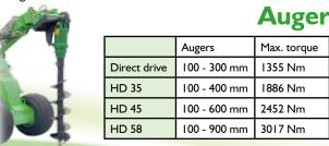
Powerful hydraulic auger with many different auger diameters to suit various tasks, be it post hole boring, tree transplanting etc. Planetary drive gives a lot of torque, replaceable teeth (tungsten teeth as standard) and pilot head enable drilling in hard ground and sandstone also. With the optional extension shafts drilling depth can be increased to max. 2,5 m.
