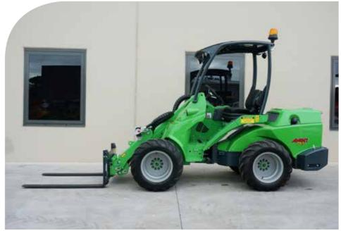
Despite the increase in power, comfort and versatility, Avant haven't compromised on safety. From the load sensor system, which provides an audible warning if the rear wheels are about to lift off the ground, to the Avant quick hitch system allowing easy, safe and fast attachment coupling, the 745 maintains both functionality and aesthetics as well as providing increased opportunity for the operator to respond
