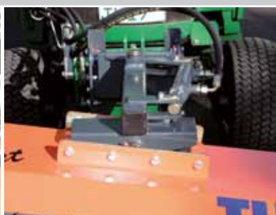
Double levelling incl. hydraulic angling
