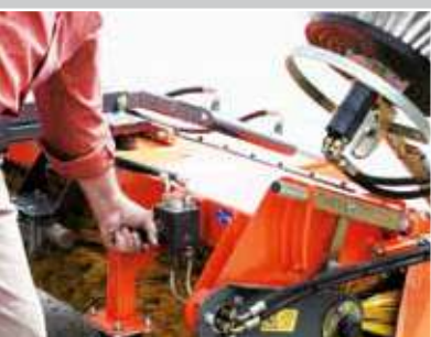
Side brush incl. speed adjustment
