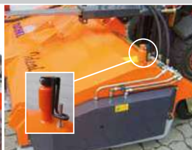
Crank handle for adjusting the floating brush
