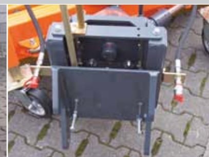
Yard loader hitch incl. levelling
