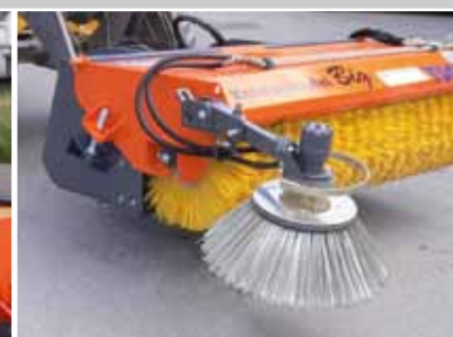
Fully adjustable hydraulic side brush (50% PP / 50% wire)
