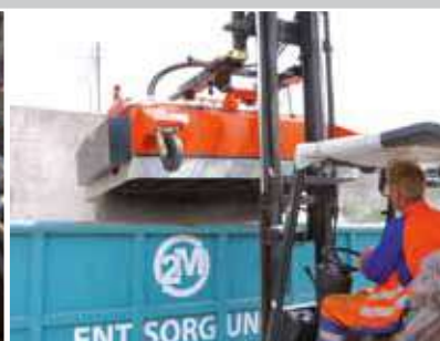
Hopper incl. hydraulic tip (standard)
