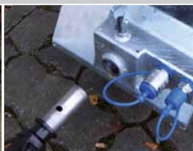
Hitch system and double-acting hydraulic connector (standard)
