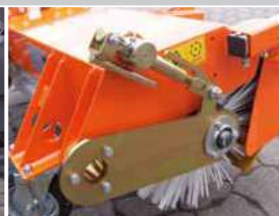
Broom adjustment via spindle
