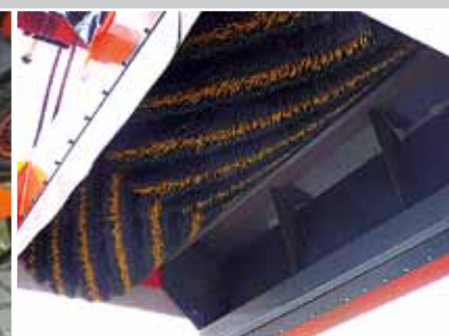
Special V-brush for sticky and fine dirt
