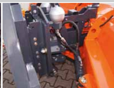
Hydraulic angling of the folding wings
