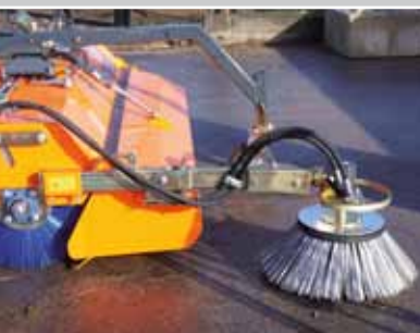
Side brush \varnothing 600 mm
