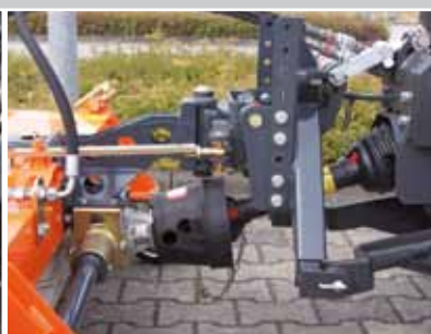
PTO-drive for 540 up to 2100 rpm
