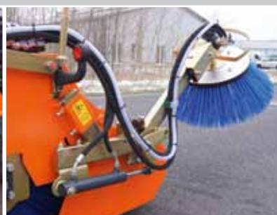
Side brush with hydraulic lifting and lowering
